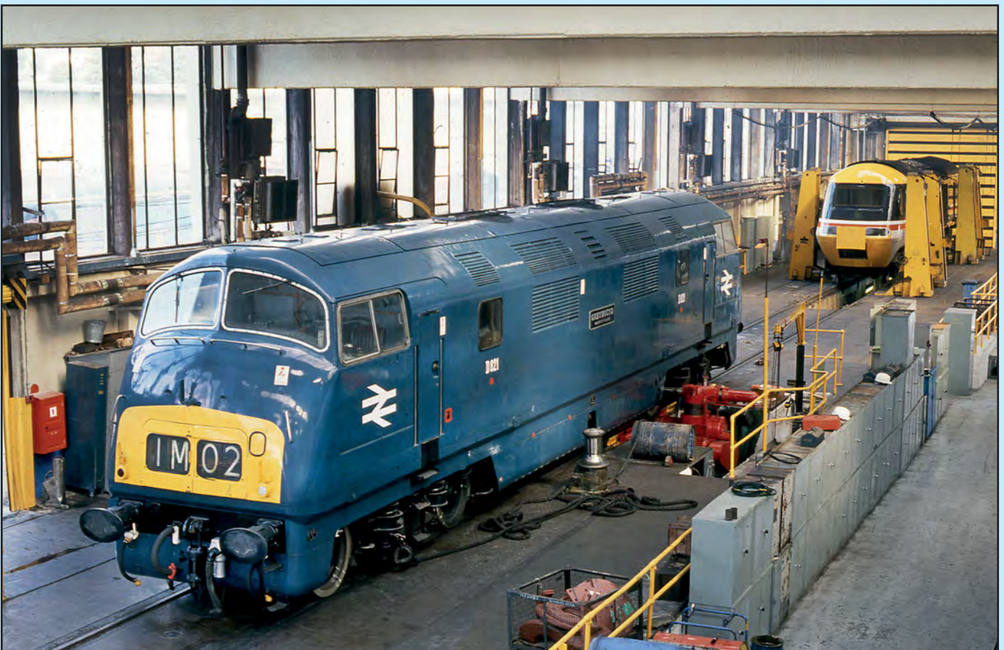
Below: After taking part in a well attended open day at Laira depot in September 1991, when D821 shared depot space with a 'Hymek' and five 'Westerns', the 'Warship' received wheelset attention on the Laira wheel lathe, which at the time was more used to dealing with HST power cars. On 28 September 1991 No. D821 still carrying its blue with small yellow warning end livery sits straddling the lathe, while a Class 43 power car stands behind about to be lifted. CJM
