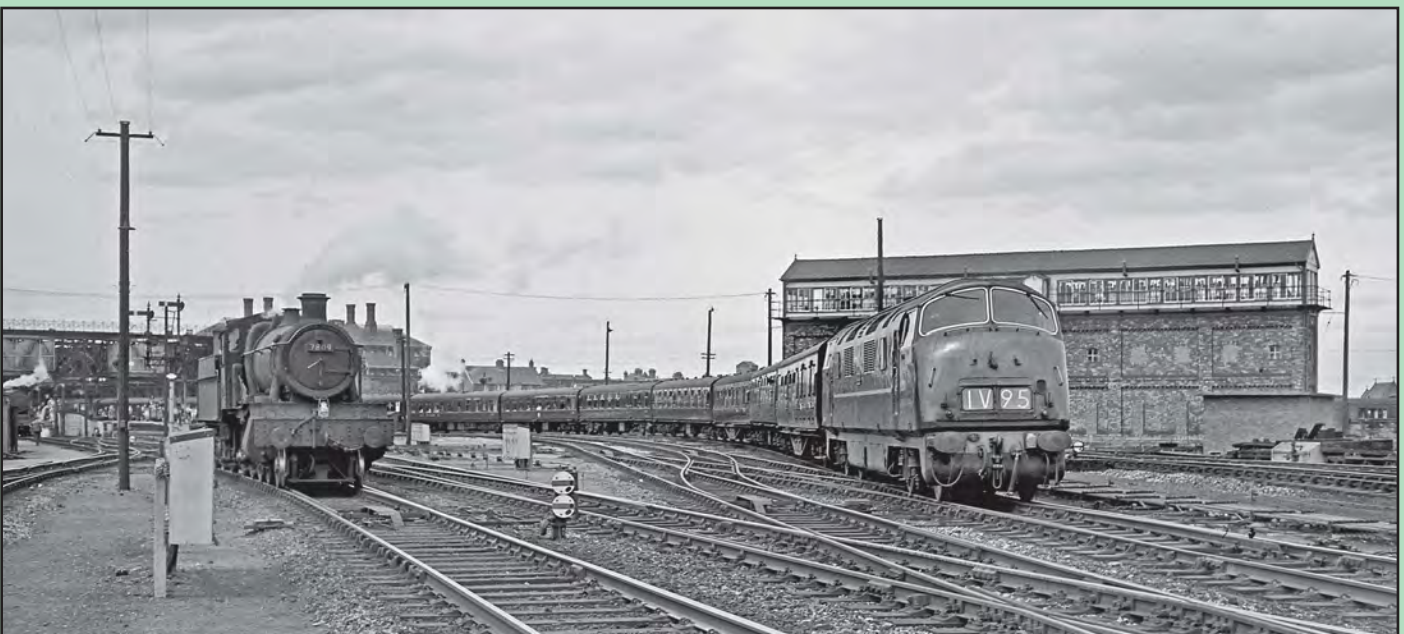
Below: In the 1960s the 'Warships', mainly the NBL built examples, were a common sight on the Western Region route to Shrewsbury. On 23 June 1962, No. D854 Tiger departs from Shrewsbury on the 12.25 inter-regional service from Manchester to Plymouth. On the left is GW-built 4-6-0 'Manor' No. 7809 Childrey Manor, which was one of the first of the class withdrawn from Shrewsbury in April 1963. John Whiteley
