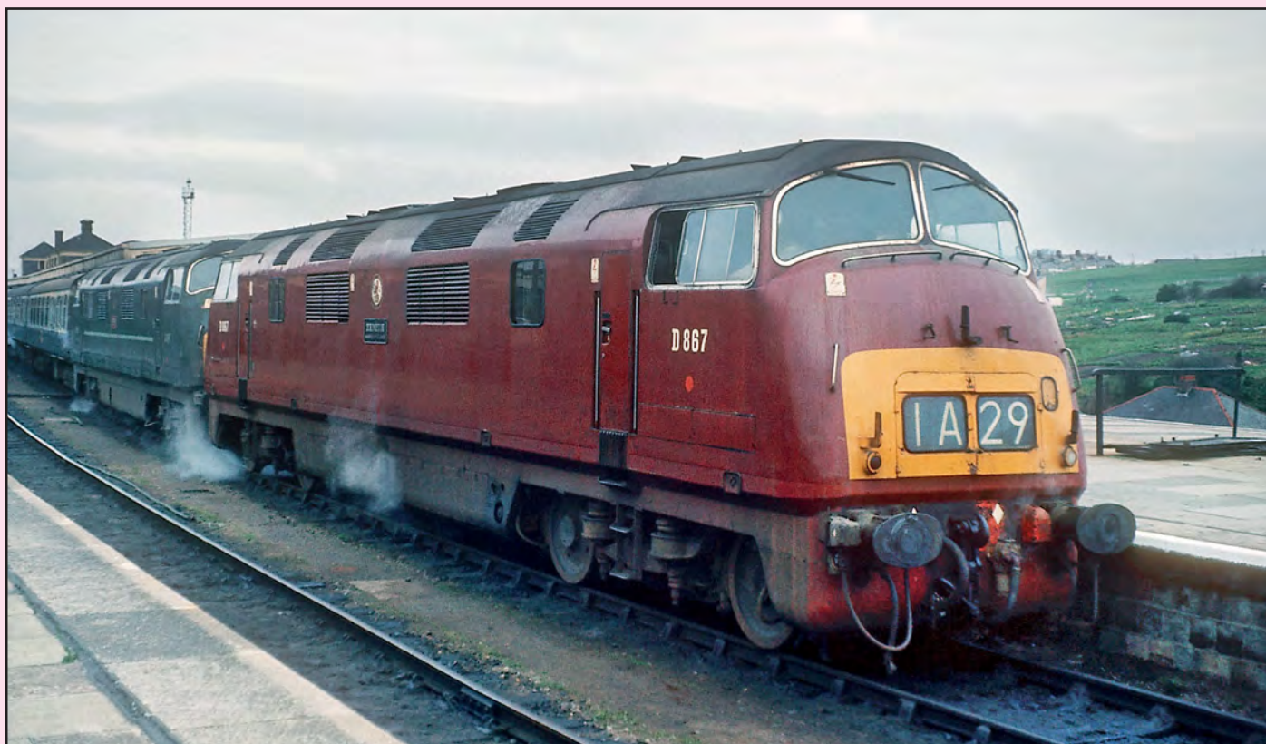
Below: Carrying maroon livery with small yellow warning ends, No. D867 Zenith operates in multiple with Green liveried with small yellow warning end No. D866 Zebra at Plymouth on 24 April 1968. The pair provide 4,400hp for the 08.30 service to London Paddington. Jim Binnie / www.dieselimagegallery.com
