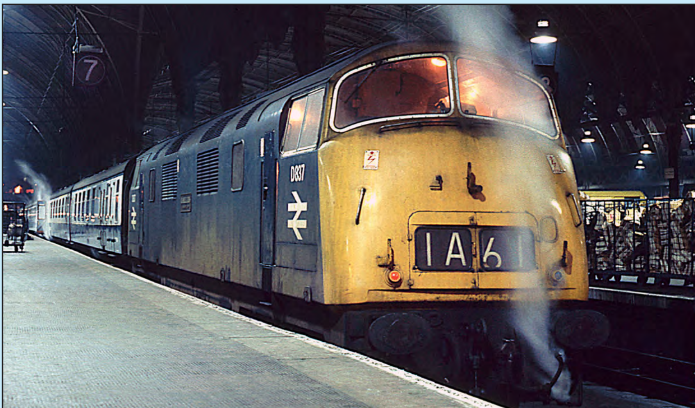
Below: A whisp of steam emitting from the nose end and between the coaches indicated the Stones train heat boiler was working on NBL No. D837 Ramillies. The loco is seen resting by the buffers at Paddington on 6 February 1970. Norman E. Preedy
