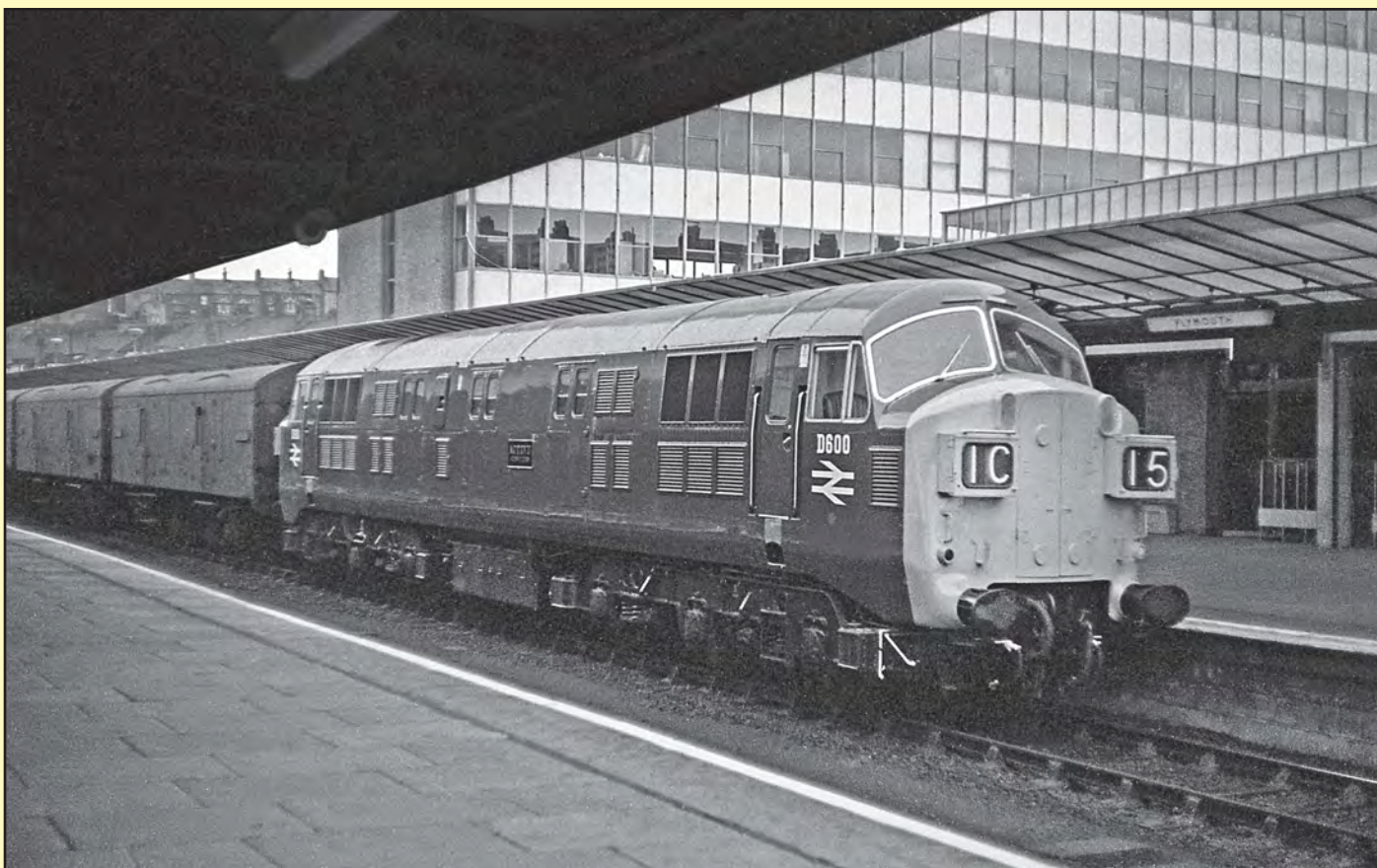
Below: On 8 May 1967, No. D600 Active was released from Swindon Works painted in full BR corporate rail blue livery, with full yellow warning ends, the only loco of the fleet to be so treated. It also sported split four character route indicators. The loco is seen at Plymouth with a van train. www.rail-online.co.uk
