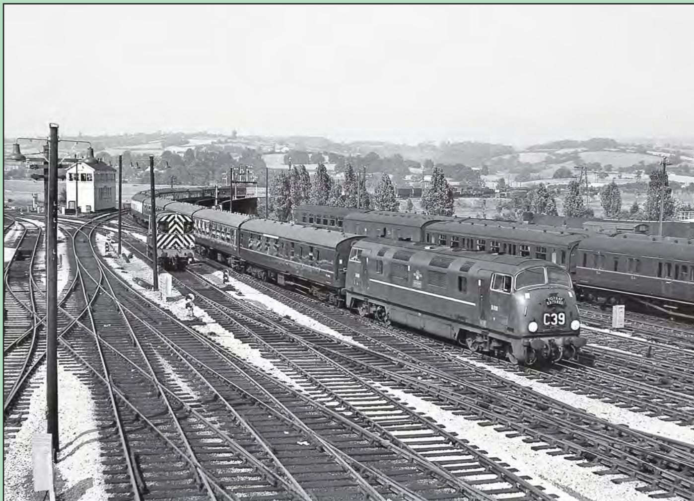
Below: Newton Abbot was one of the prime locations in the West Country to see and record all of the Western Region diesel-hydraulic classes. Adjacent to the station was a sizeable depot and workshops which over the years was one of the main servicing and repair depots for the production 'Warship' fleets. On 25 July 1962, No. D810 Cockade arrives at Newton Abbot powering the westbound 'Torbay Express'. On the left of the train one of the depots 0-6-0, later Class 08 shunting locos can be seen which would have been operating station pilotage duties. John Whiteley
