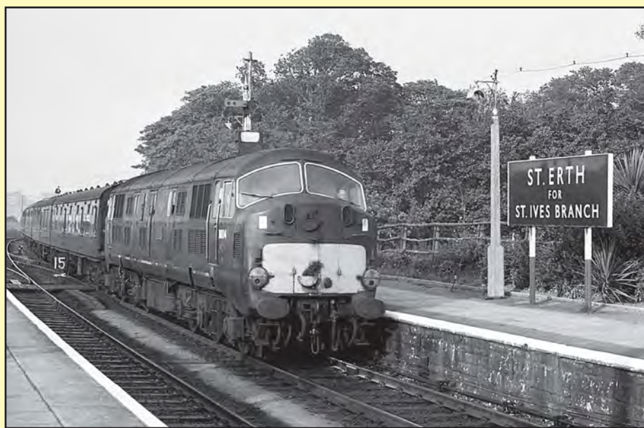
Right Middle: Slowing for the station stop at St Erth and providing a connection with the St Ives branch train, D600 'Warship' No. D604 Cossack powers a Penzance bound service on 25 May 1965. By this time the deployment of NBL A1A-A1A 'Warships' in the far west was reducing, with production NBL B-B 'D800s' and BR D1000 class locos operating the majority of services. K Nuttall / www.colour-rail.com
