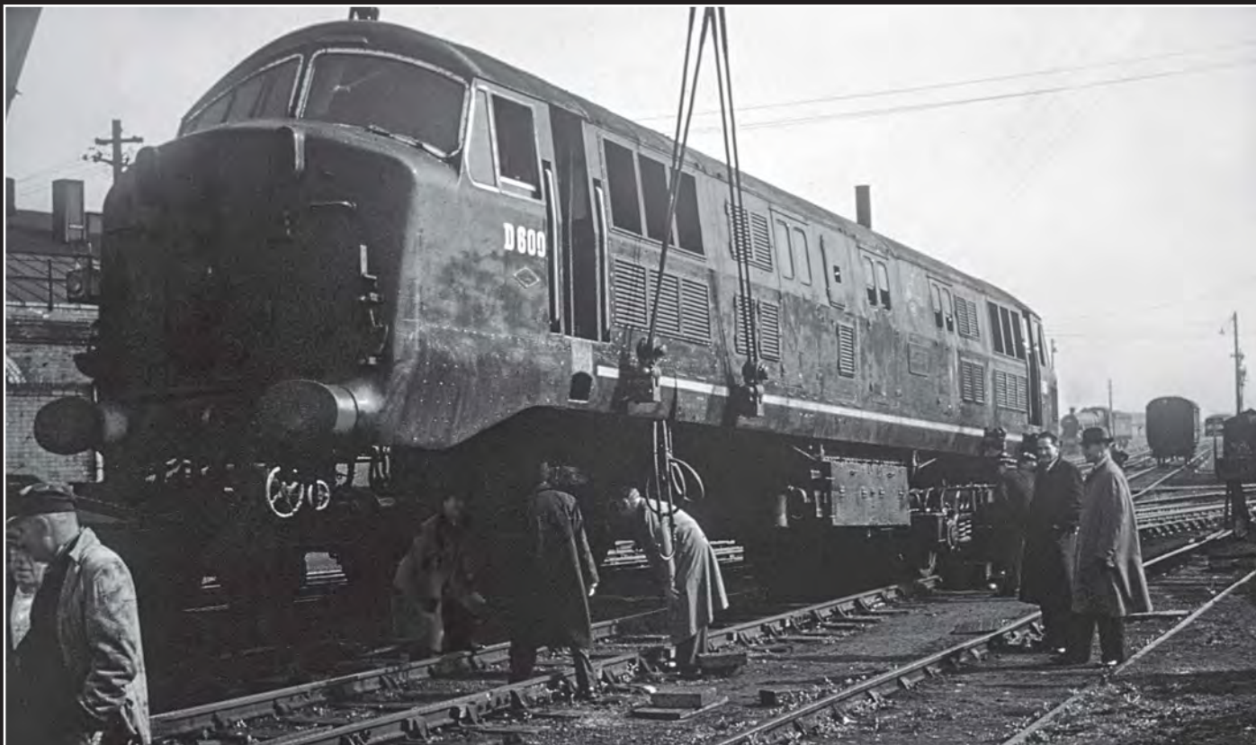
Above: D600 Active seems to have had a slight problem. In this image dated March 1960 the loco has one end supported by a crane, showing the dual lifting lugs located on either side of the loco at both ends. The bogie appears to have been removed and attention given to the underside equipment. CJM-C
