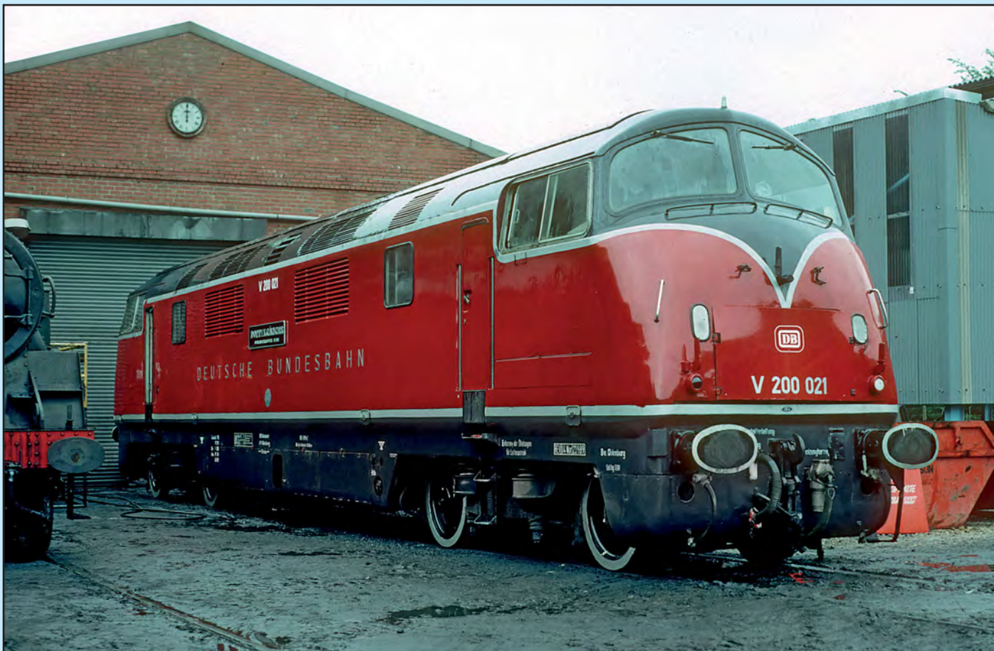
Above: In summer 1990 a little fun was had by the Diesel Traction Group, when they repainted No. D821 into Deutsche Bundesbahn livery and renumbered it as V200 021 with the nameplate Doppelganger. Even the front end was modified to resemble the German loco! No. V200 021 is seen at Grosmont shed on 7 July 1990. Paul Winter
