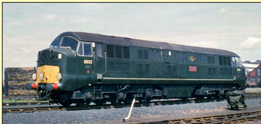
Right Below: Photographed at Swindon Works on 18 June 1962, No. D602 Bulldog shows the small yellow warning end which it gained just nine weeks prior. The record books show that the D600s spent a considerable amount of time at Swindon Works receiving either classified or casual repairs during their short operating life. K Nuttall / www.colour-rail.com
