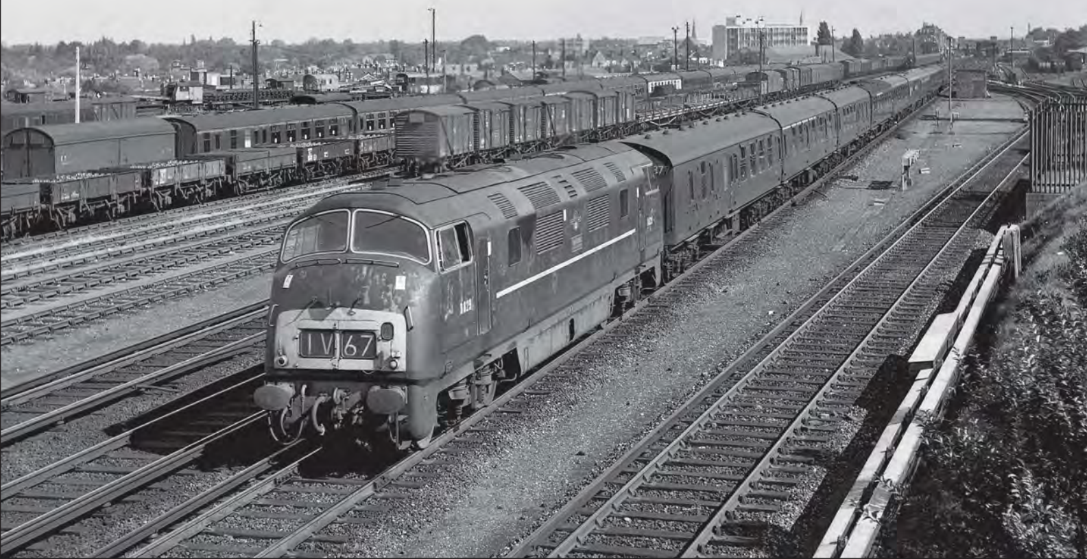
Above: Passing Woking Junction, south of Woking station, where the Guildford line diverges from the L&SWR main line, and passing the huge yard complex on both sides of the main line, 'Warship' No. D829 Magpie powers the 11.00 Waterloo to Exeter St Davids on 13 September 1964. The L&SWR main line was four track section through to Worting Junction and was arranged with the fast lines in the middle of the formation and the slow tracks on the side. Brian Stephenson
