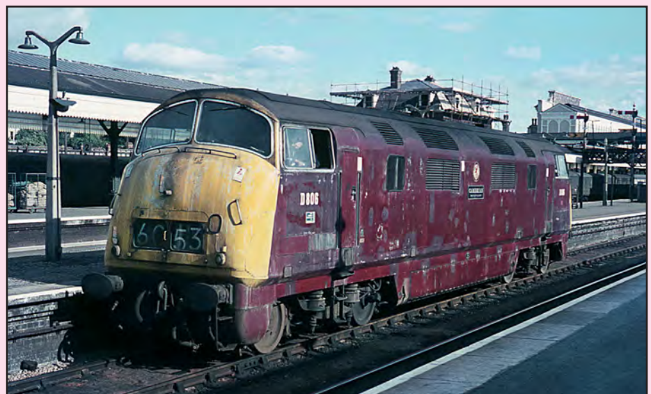
Right Below: By the early 1970s, the remaining maroon 'Warships' were looking in a very dilapidated condition, with faded yellow ends and patched bodywork, where filler had been applied to fill rust spots and painted over with a close colour. Looking well work stained, No. D806 Cambrian is seen at Exeter St Davids on 9 July 1970. In March 1971 the loco was repainted in rail blue during an intermediate overhaul at BREL Swindon. The loco was withdrawn on 1 November 1972. Norman E. Preedy
