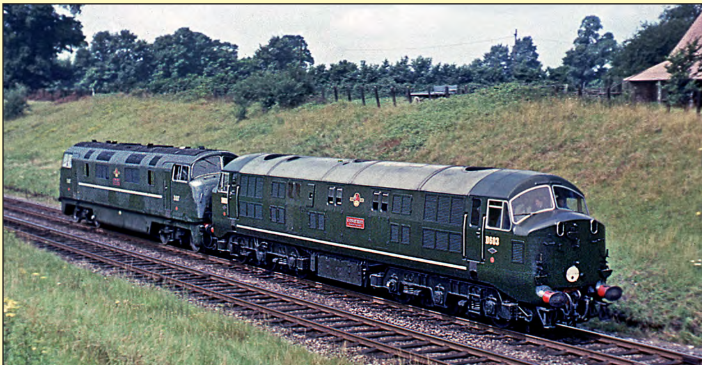
Below: It is not often that pictures turn up showing the two different designs of 'Warship' together. In this view recorded in the summer of 1961, we see NBL D600 'Warship' No. D603 Conquest, coupled to BR Swindon built D800 'Warship' No. D807 Caradoc. The differences in length and green livery style are quite noticeable. www.colour-rail.com
