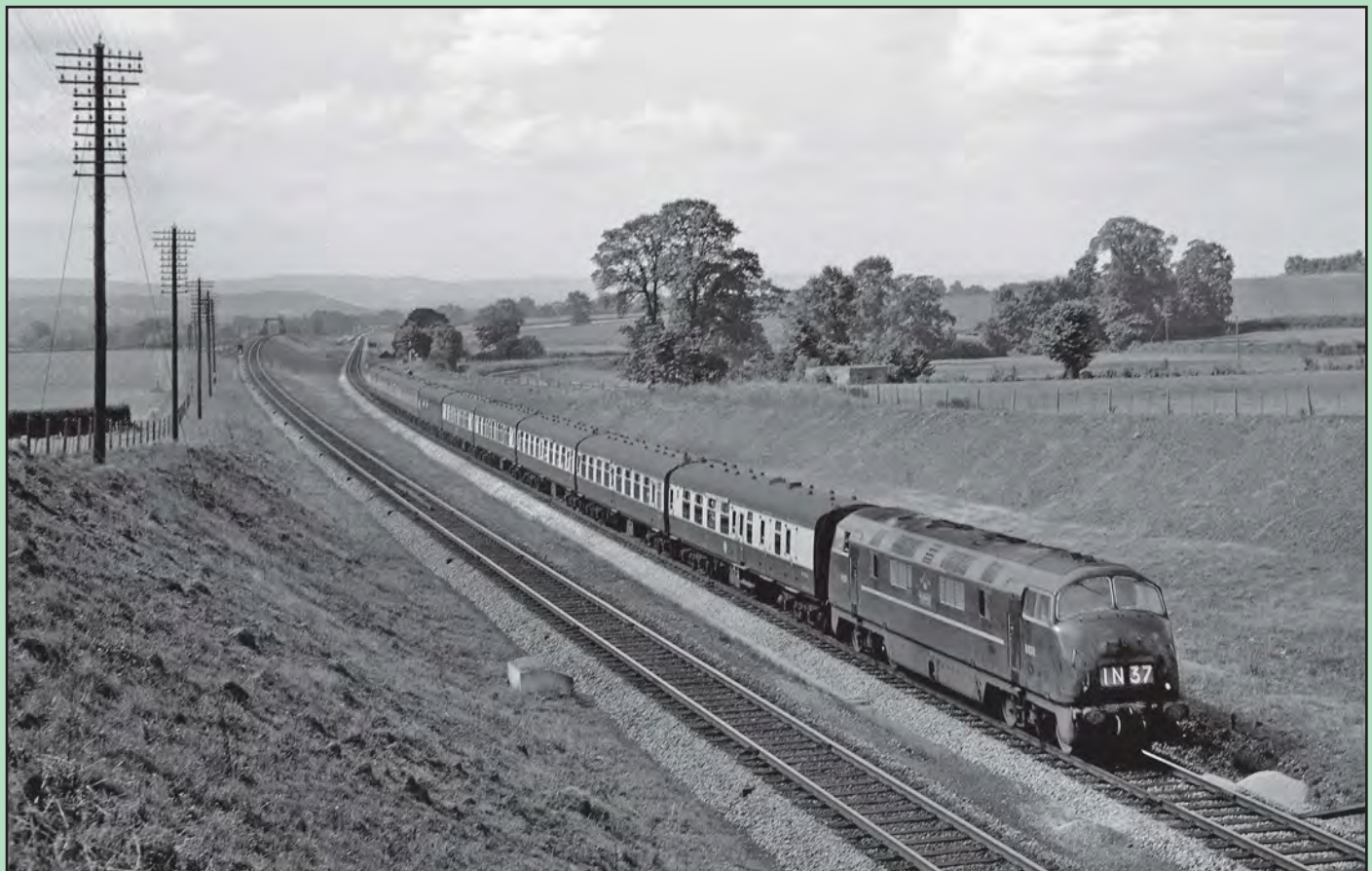
Below: The unique No D830 Majestic, fitted with a pair of Paxman 12YJXL 'Ventura' engines, passes Cogload Junction nearing Durston north of Taunton on 17 August 1961 powering 'The Devonian' from Paignton bound for Bradford. The 'Warship' would have been replaced by either steam power or a diesel-electric at Bristol. M. J. Fox / Rail Archive Stephenson
