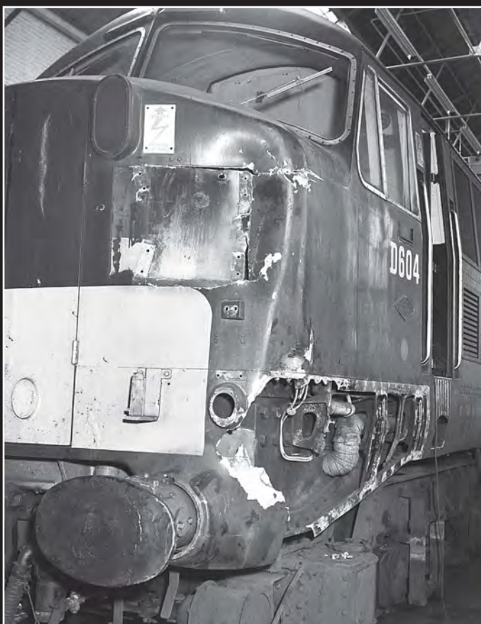
Below Left: North British A1A-A1A No. D604 Cossack received front end and side swipe damage in February 1967, just a couple of months after it received four-character route indicator boxes. The damage reported to have been received at Laira depot was repaired between 2-22 March 1967 at Swindon Works. CJM-C
